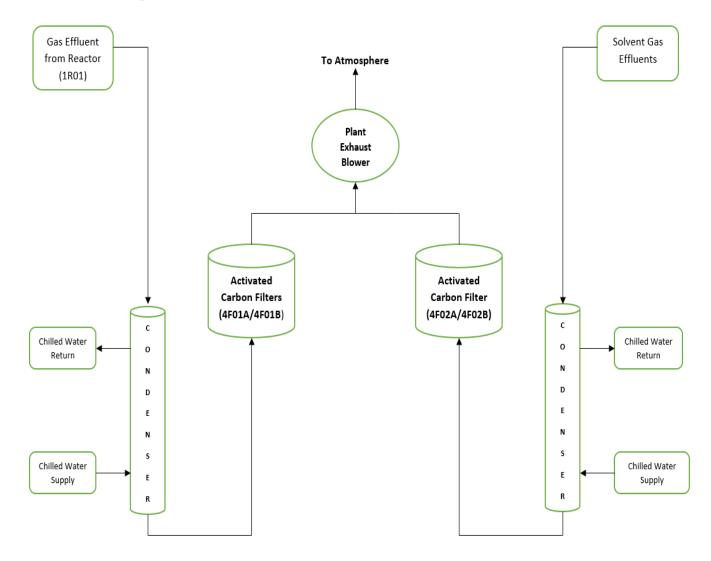
7.5.3.1 Process Diagram for the Treatment of Waste Gases
